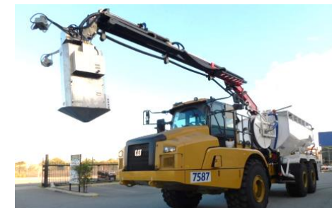
Robotic explosive placement
