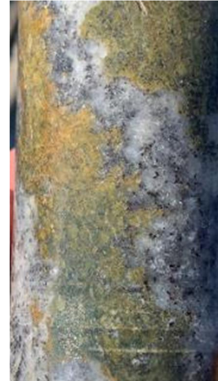
P2 (Red Stock) Higher grade +20 g/t Au UST zone East Zone (RC10-423; 873m)
