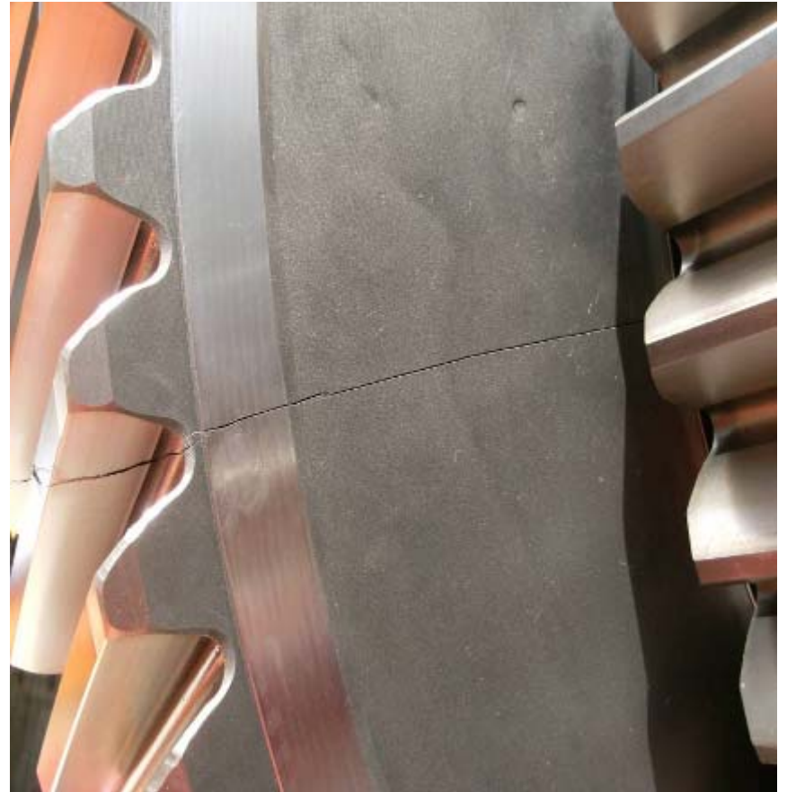
Cracked Mill Gearbox
