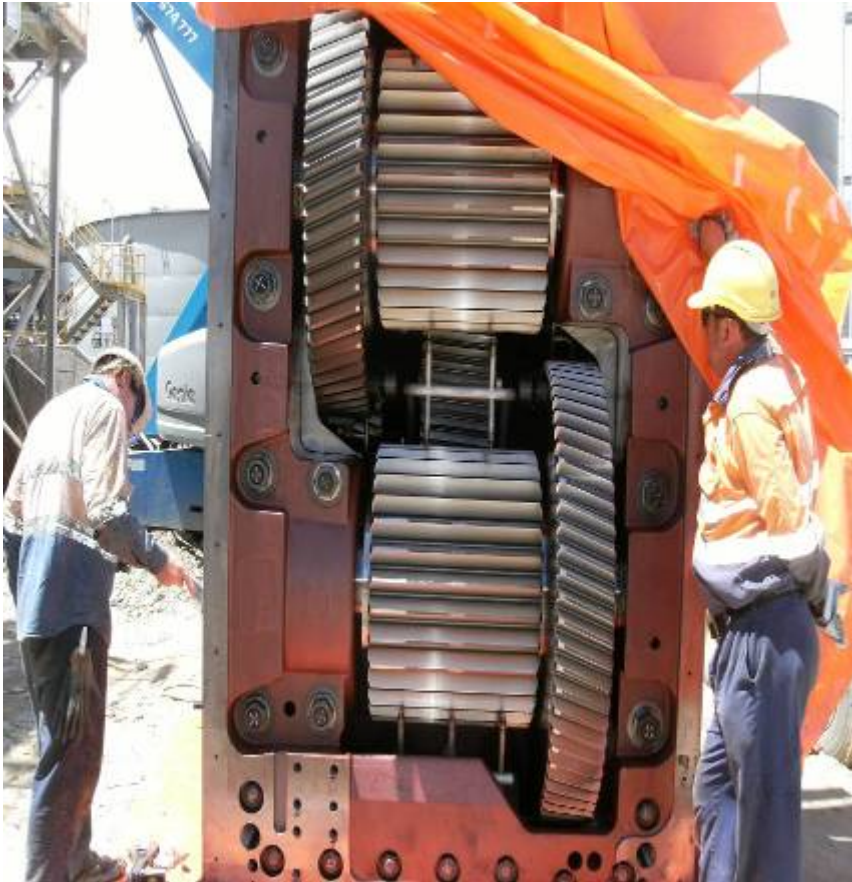
Cracked Mill Gearbox
