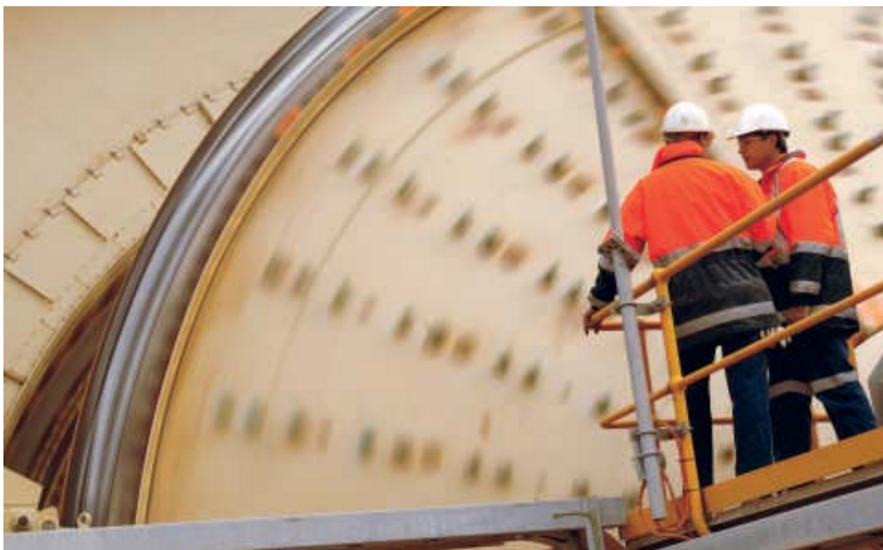
Frank Reid and Sam Booth inspect the Semi-Autogenous Grinding Mill at Telfer.
