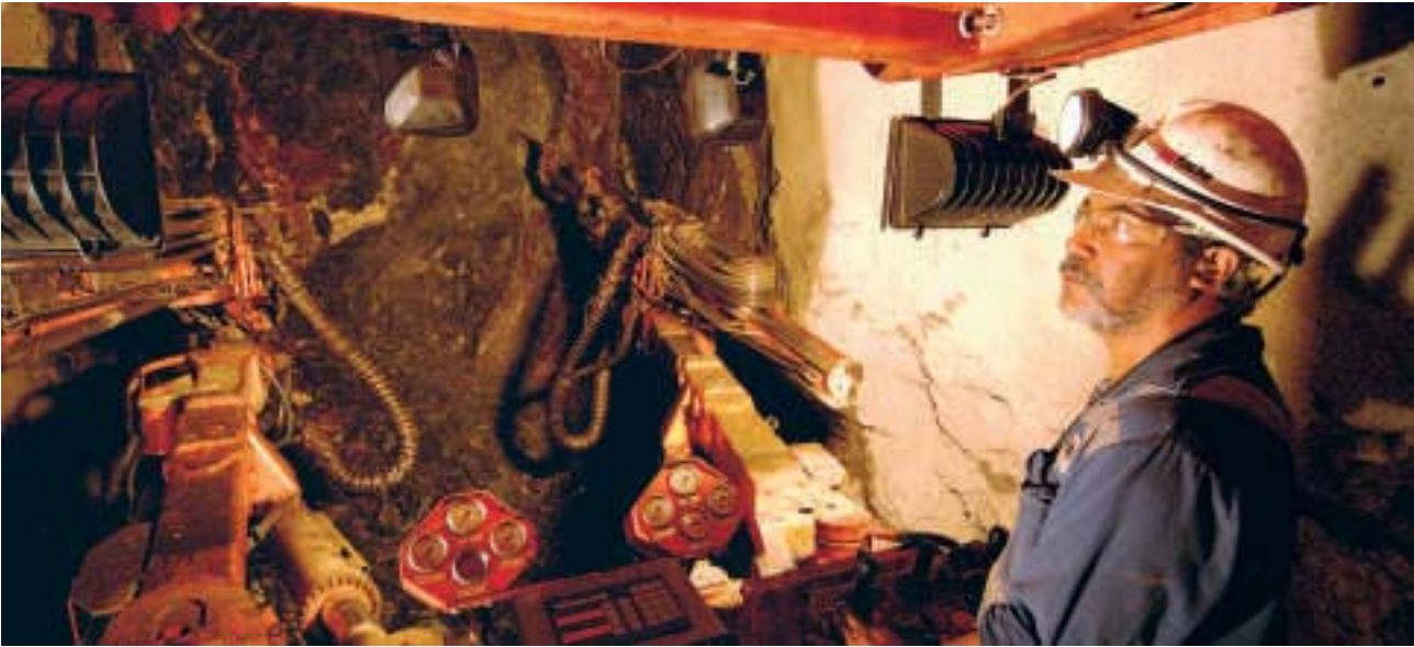
Roche Mining Jumbo Operator, Des Motlap, boring an ore development heading at the Cracow underground mine.
