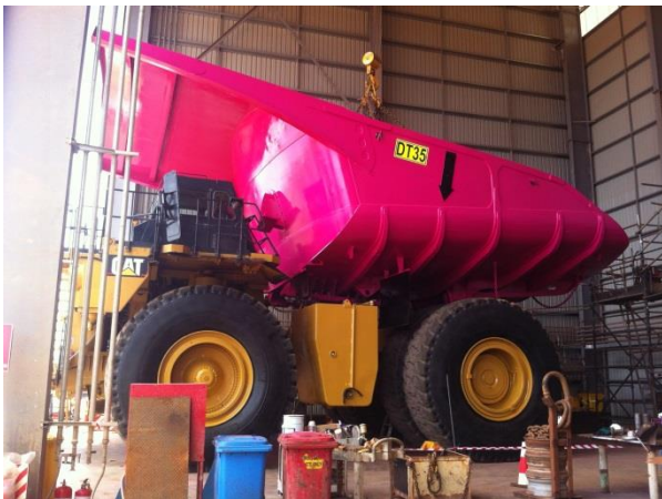
The repainted CAT 793D tray is lowered onto its wheels.
