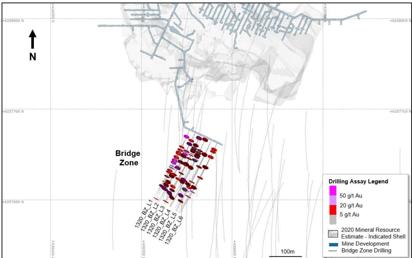
Figure 13. Schematic plan view map of the Bridge Zone – Phase 1 drilling showing the location of the drill fans and previous drilling in the Bridge Zone relative to the mine development and the 2020 Mineral Resource Estimate area.
