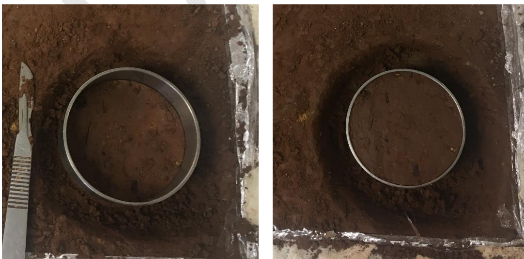
Figure 4: Coring specimen from block sample
