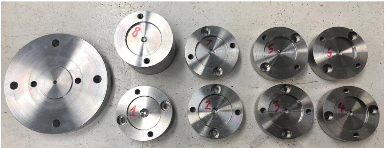
Figure 5: Tamper dismantled with various spacers
