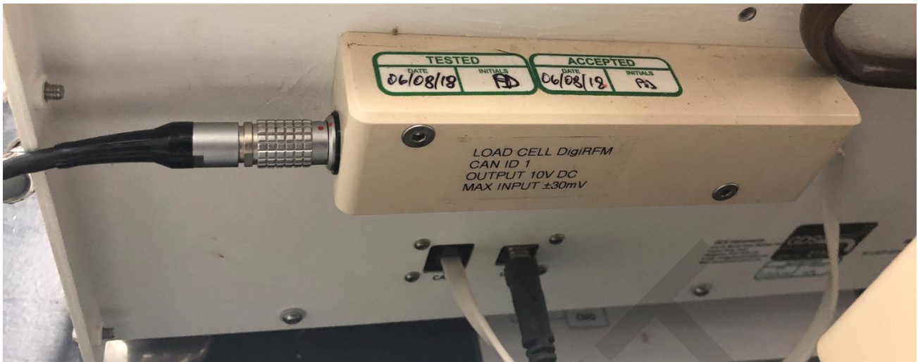
Figure 2: View of DigiRFM servo-controller mounted at the back of the load frame
