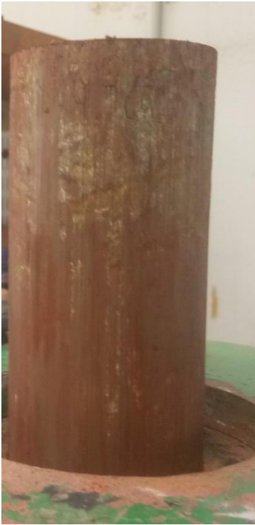
Figure 5: Sample extruded for triaxial testing
