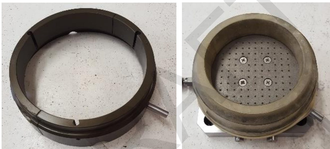
Figure 1: GDS specimen preparation mould (left) and DSS mould while suction is applied (right)
