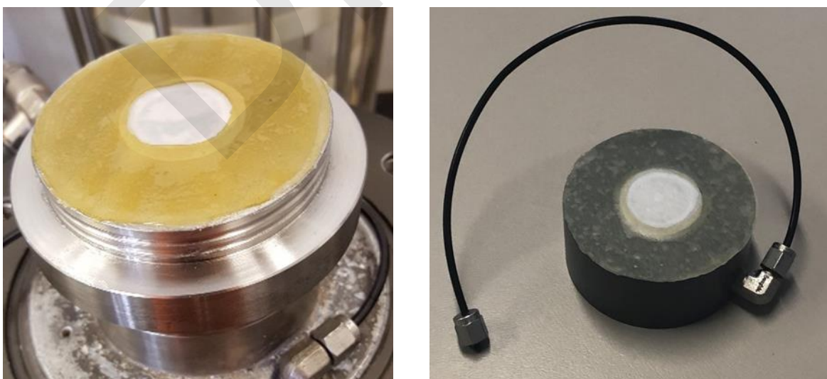
Figure 4: Modular base with lubricated end platens (left) and top cap with lubricated end platens (right)
