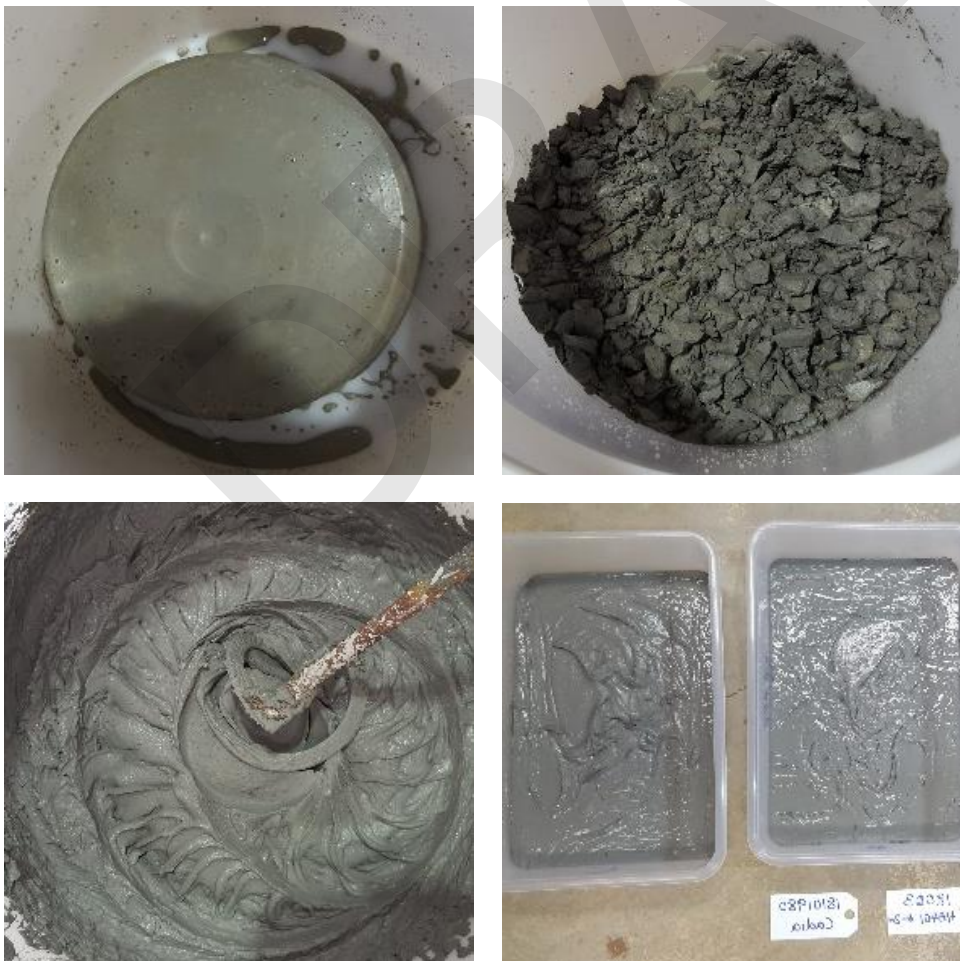
Figure 1: Sample prepared as thick slurry
