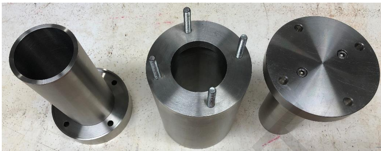
Figure 2: View of different components of compactor: mould base platen with the inner sleeve (left), outer sleeve (middle) and adjustable height tamper with top platen to allow controlling the height (right)
