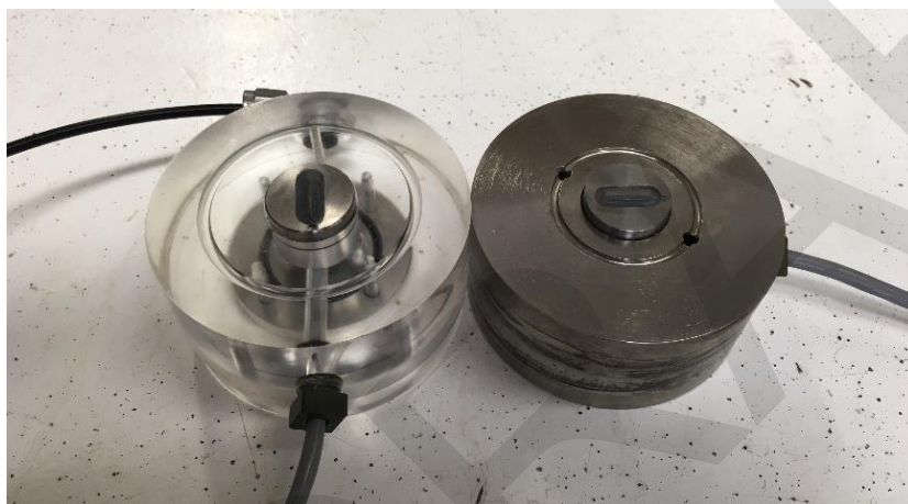
Figure 3: Set of caps with bender elements
