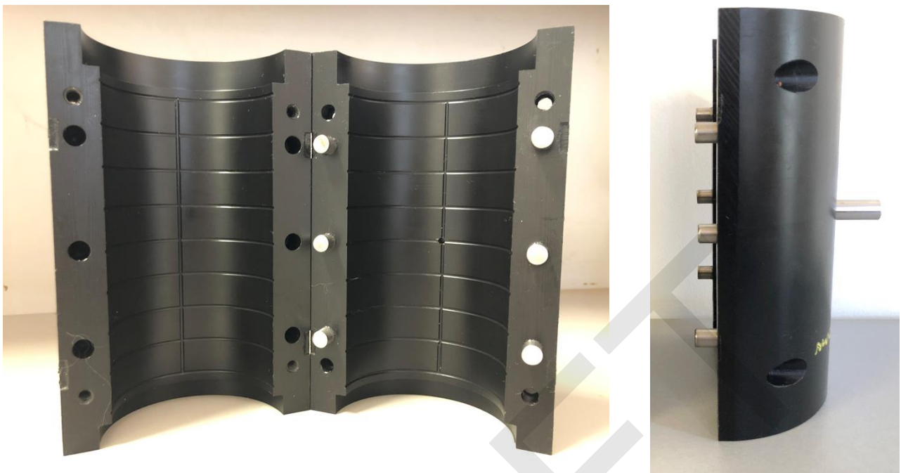
Figure 2: Split mould internal (left) and external view (right)
