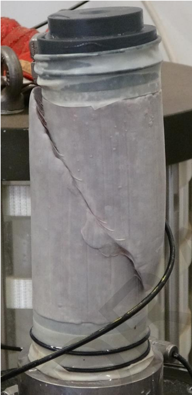
Figure 2: End of test typical deformed specimen with a slip plane
