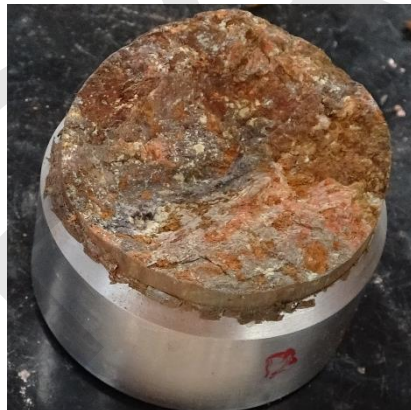
Figure 6: Sample extruded into a stainless-steel ring for DSS and CRS testings
