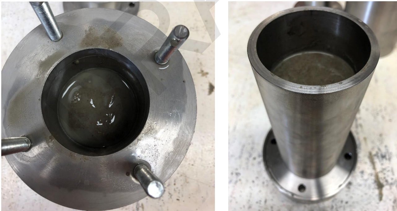
Figure 8: Water at surface of sample at vibration of mould (left) and specimen after compaction inside inner sleeve
