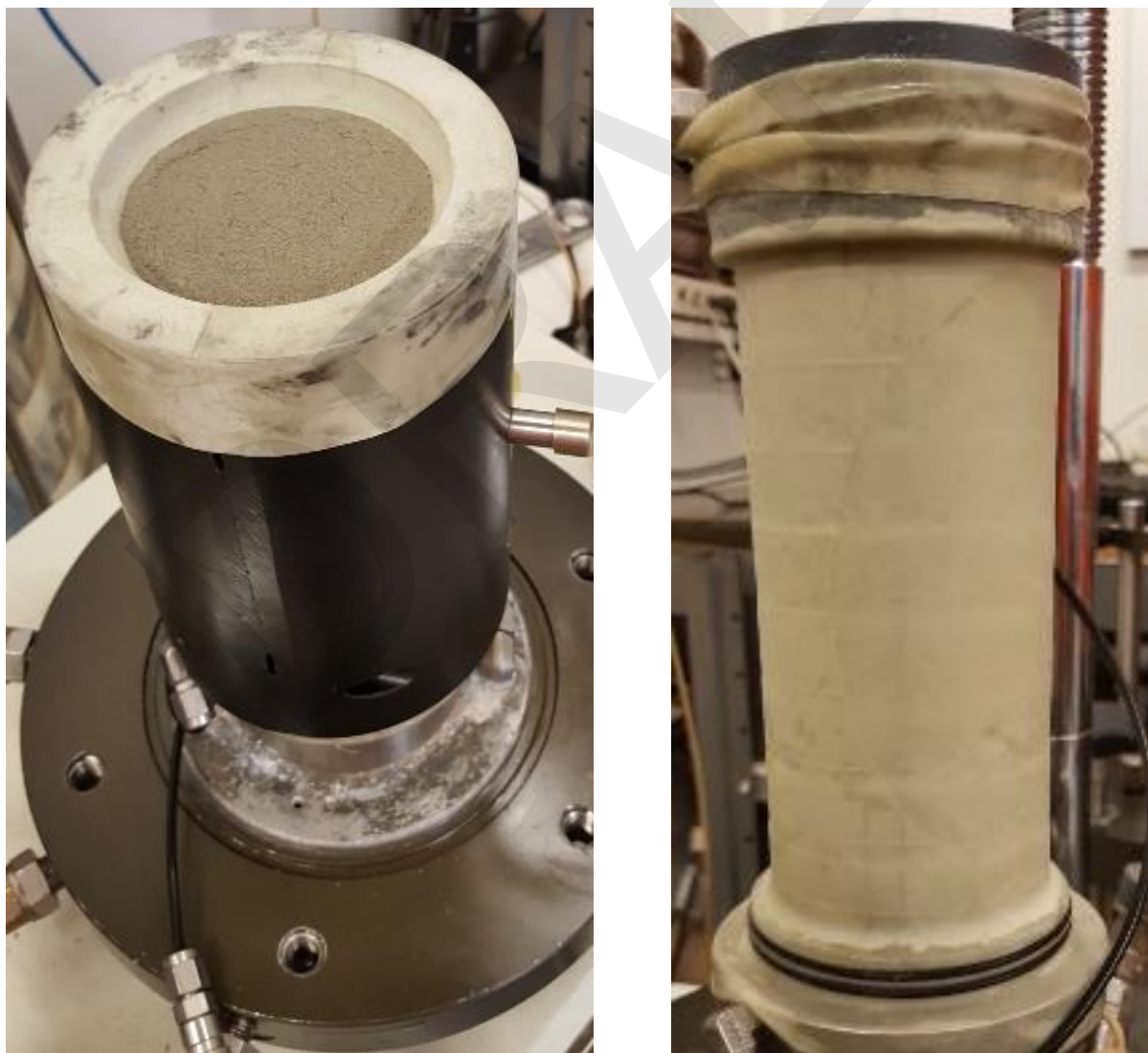
Figure 7: Tamped specimen prior placement of top cap (left) and with top cap after removal of split mould (right)
