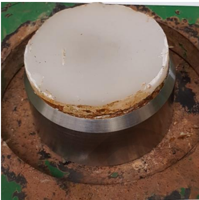
Figure 6: Sample extruded into a stainless-steel ring for DSS and CRS testings
