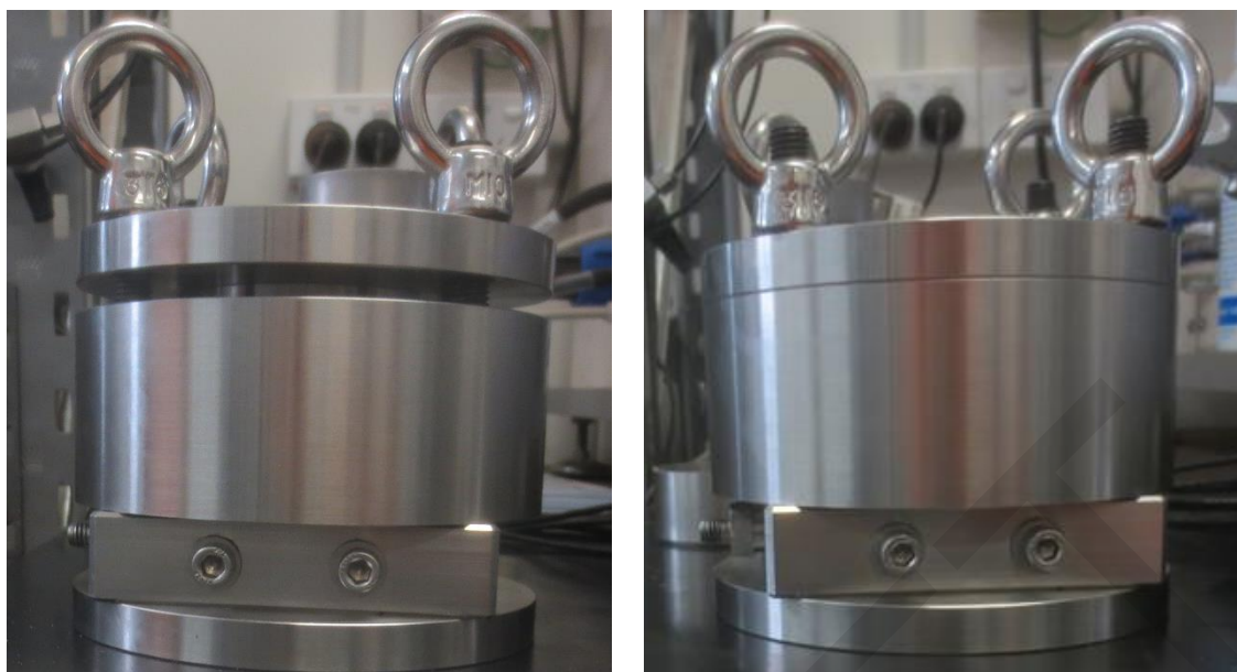
Figure 4: DSS specimen inside compactor mould: before compaction (left) and after compaction (right)
